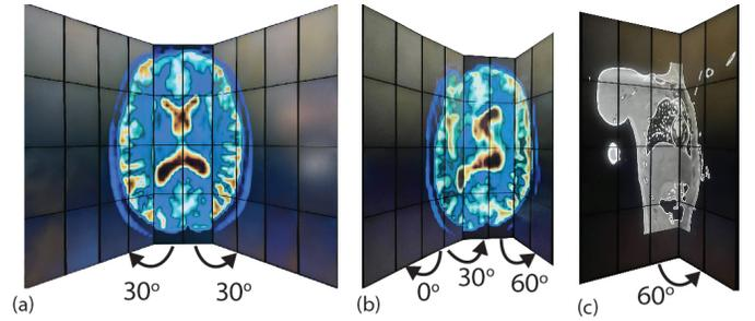
Fig. 8: (a) A "U"-shaped layout resulting in a center (flat) cutting plane and two planes rotated at 30°. (b) An example where the column-pairs from the center are rotated at 30° and 60°, respectively. (c) Volume rendering of a full-body CT data, showing a limitation where rotating the plane  $> 60^\circ$  exceeds the volume bounds.
