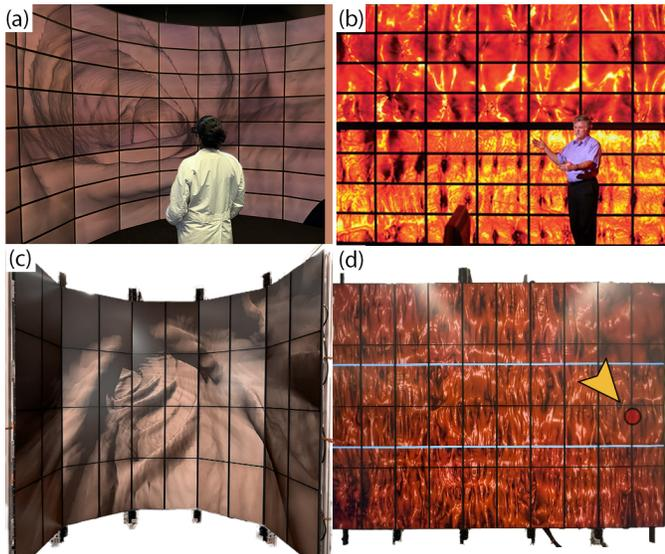
Fig. 4: (a) Immersive Virtual Colonoscopy (VC) visualized in a curved display facility. (b) 2D view of the flattened VC data visualized in a planar display facility. The reconfigurable display layout of the FlexiCAVE can facilitate both immersive and flat VC visualization techniques. (c) Immersive VC of the user-selected region (red cursor pointed by the yellow arrow) from the flattened colon view, shown in (d).
