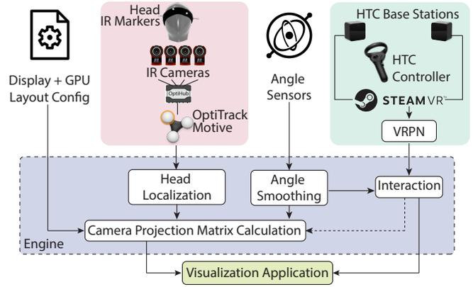
Fig. 3: System design of our modular Engine framework for the multi-node and multi-GPU FlexiCAVE setup. Using display and system configurations, along with user and controller tracking, Engine updates camera views and visualizations, abstracting them from the application design.
