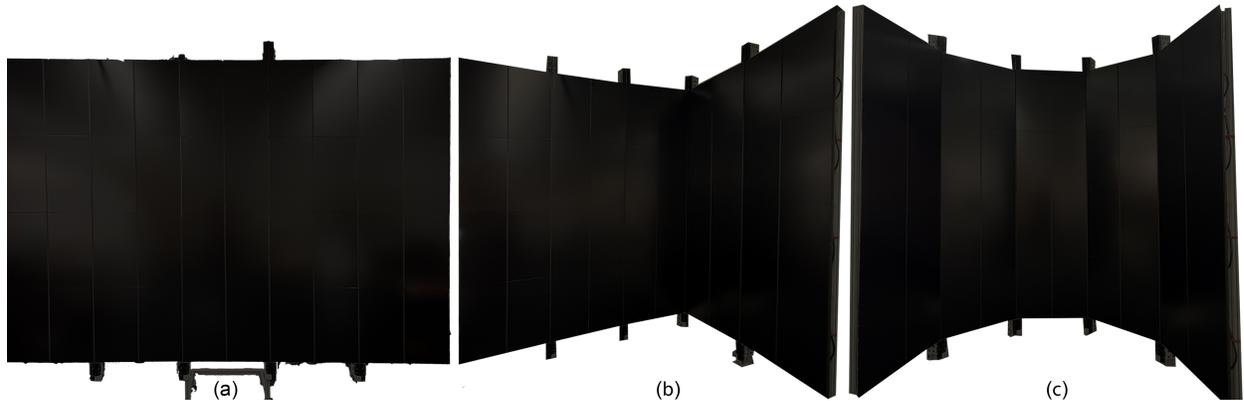
Fig. 1: The FlexiCAVE display facility can be dynamically transformed into various display configurations by adjusting the hinged display columns into many various configurations, such as: (a) flat, (b) flat two-sided, or (c) curved.
