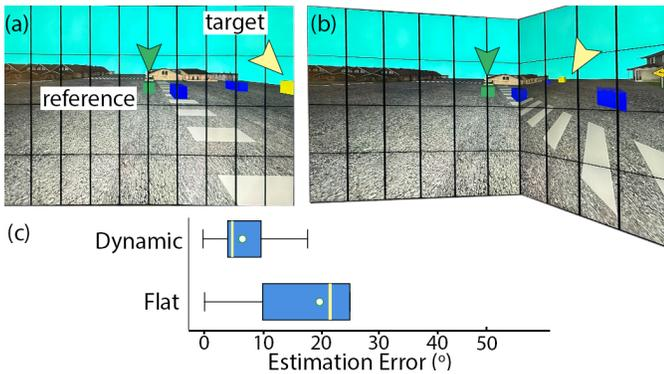
Fig. 6: Direction perception study for (a) the flat layout (target at  $45^\circ$ , 2m from reference), and (b) an example user-set dynamic layout (target at  $30^\circ$ , 6m from reference). (c) Angle estimation error for both layouts, with the white bar and dot representing median and mean errors, respectively.
