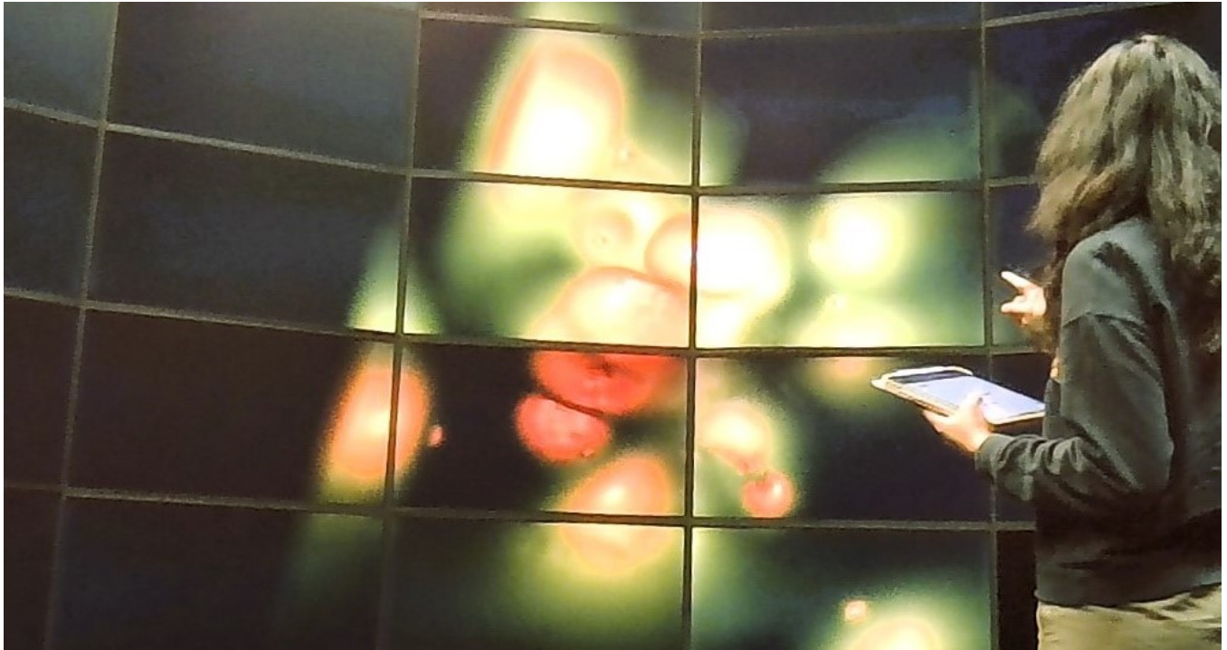
Figure 1: A user investigating the volume visualization of the electron potential of an iron protein molecule on Silo - an immersive facility - along with the interaction interface on an iPad device.
