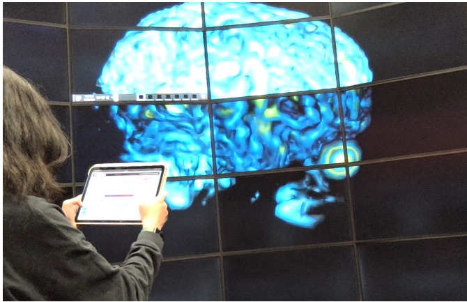
Figure 4: A user interacting with the MRI scan of a human brain, dynamically adjusting the transfer function.
